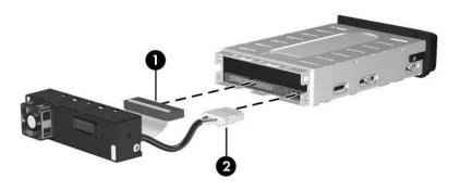
Connecting the Hard Drive Carrier Rear Panel
